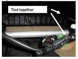
4. Pop up rear plastic frame holders and carefully remove seat controller with its frame
