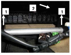
6. Take seat Controller out from its frame by gently pushing left and right security clips
