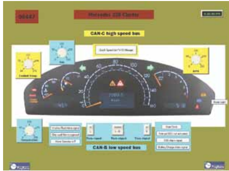
An Instrument Cluster is being tested by a proprietary CAN base tester
