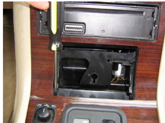
4. Take out L-R vertical start-headed screws
