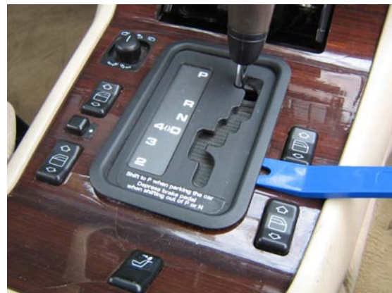
6. Carefully remove frame
