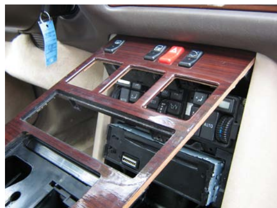
8. Remove upper wood frame
