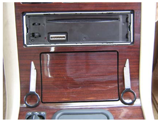
2. Remove radio by using the right tool
