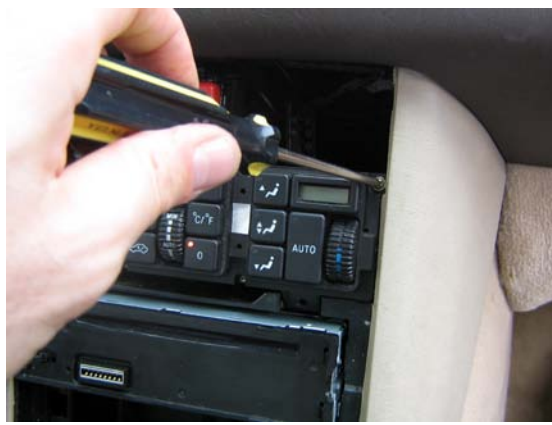
10. Unscrew, remove and disconnect Unit
