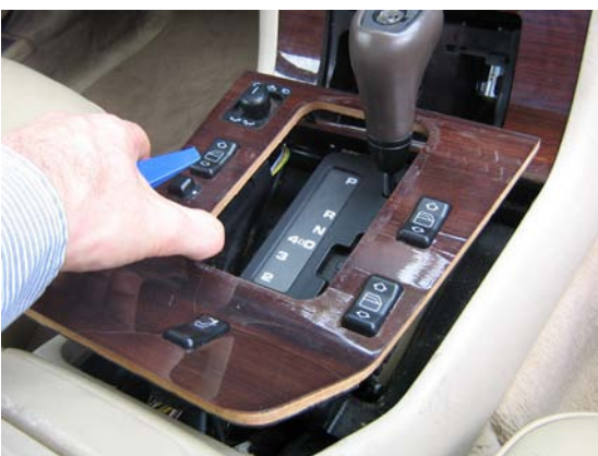
7. Remove lower wood frame
