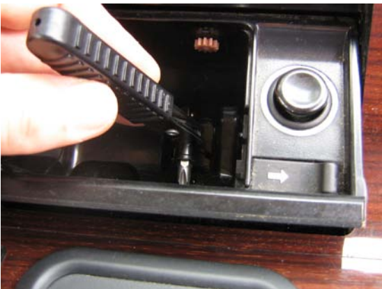
3. Loosen inside screw and remove cover
