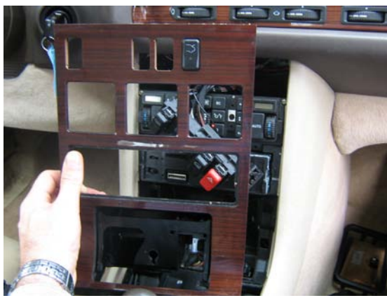
9. Disconnect Switches and connectors
