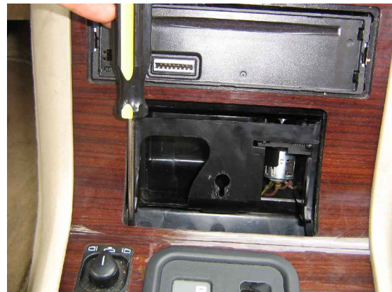
4. Take out L-R vertical start-headed screws
