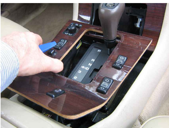
7. Remove lower wood frame
