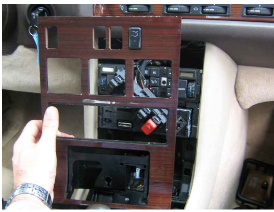
9. Disconnect Switches and connectors
