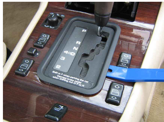
6. Carefully remove frame
