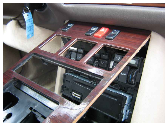
8. Remove upper wood frame
