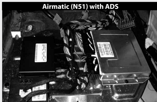
Unscrew 3 bolts holding the aluminum bracket
